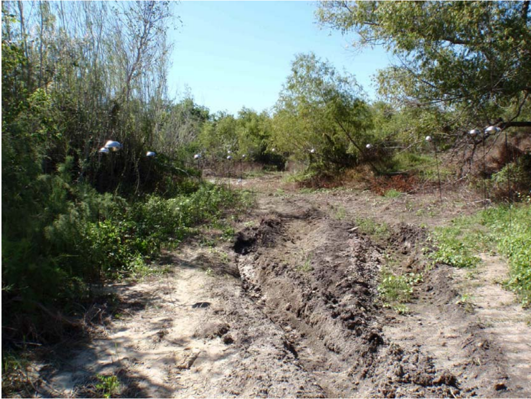
Figure 3. Photograph of the passive samplers positioned at the North Pit. Summa canisters were positioned at each end of the line of sampler housings. They are not visible on this photo.
