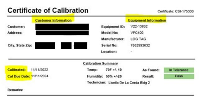
Figure 3-2. Example of a data logger Certificate of Calibration.
