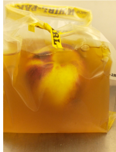
A whole peach being tested for Listeria monocytogenes contamination. The peach is immersed in Buffered Listeria Enrichment Broth (BLEB), which selects for the growth of the bacterium Listeria in foods. (Chris Malota, 2022. © DSHS.)
