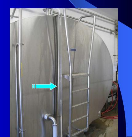
To use the internal measuring rod, first remove and wipe clean with a clean single service paper towel
