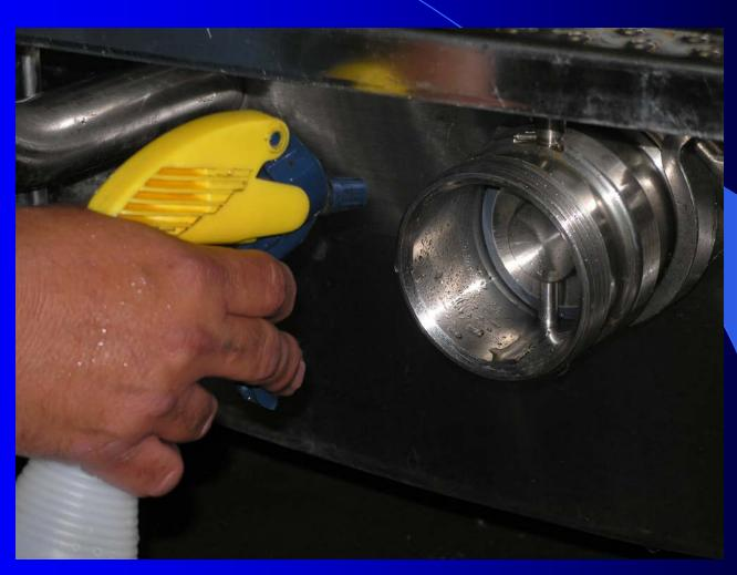
Remove the cap from the milk transfer hose and store to protect from contamination
