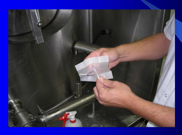
Insert the needle through one of the unused sampling guide ports
