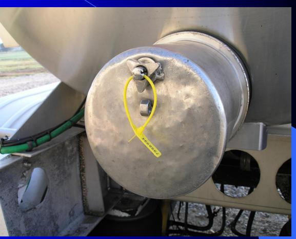
Seals must be numbered and tamper-evident. They may be plastic, pressed metal, or wire cable.
