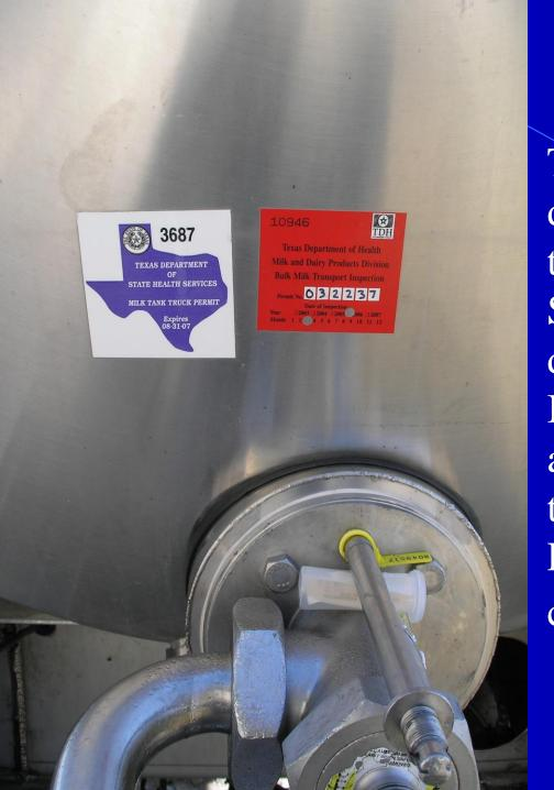
Tanker Permit and Inspection decals should be located at the rear of the tanker. Note: Some states have only ONE decal that doubles as both Inspection and Permit. If you are uncertain whether or not a tanker displays the proper Permit or Inspection decal, contact your supervisor.
