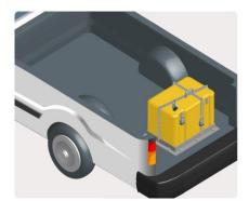
2. You store the gauge or transportation case containing the gauge in a locked trunk, camper shell, van, or other similar enclosure. You physically secure it to the vehicle by a chain in such a manner that one would not be able to open the case or remove the gauge without removal of the chain or cable. After you properly secure the transportation case, you will have to block and brace it.
